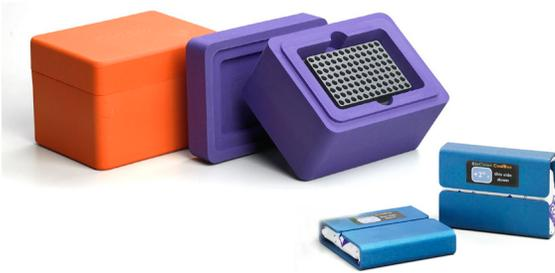
**CoolBox MP System** is an ice-free cooling or freezing container that accommodates all CoolSink and CoolRack plate modules. The reusable cooling cartridge will provide up to 10 hours of <4°C cooling while ensuring temperature uniformity across all wells of the plate. Place dry ice in the CoolBox instead of the cooling cartridge and obtain hours of -78°C freezing in a compact, portable workstation.
