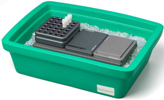
**Cooling:** Place the ThermalTray platform into a pan of ice and place the CoolSink or CoolRack modules on top. Units will equilibrate to less than 2°C in approximately four minutes. Assembly will ultimately equilibrate to approximately 1°C and hold that temperature as long as there is ice in the melted ice water (10-12 hours).
