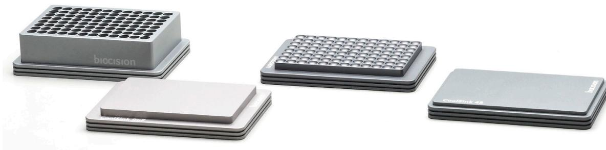
**CoolSink thermo-conductive** plate holders provide temperature-equalizing interface between plate and temperature sources such as ice, dry ice, incubators, hot plate and water baths. The novel alloy rapidly adapts to source temperature and ensures uniformity across all wells – eliminating edge effect.
