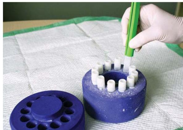
BioCision's CoolCell alcohol-free cell freezing containers ensure standardized controlled-rate  $-1^{\circ}/\text{min}$  cell freezing in a  $-80^{\circ}\text{C}$  freezer—without alcohol or any fluids.
