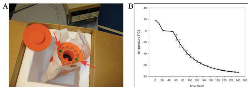
Figure 1: Freezing rate determination of an alcohol-free freezing device; A: experimental set-up, thermocouples in 2 ml cryovials were placed in the freezing-device in secondary packaging in a dry ice box. B: freezing rate of 2 ml cryovials within alcohol-free freezing device. Error bars indicate standard deviation.
